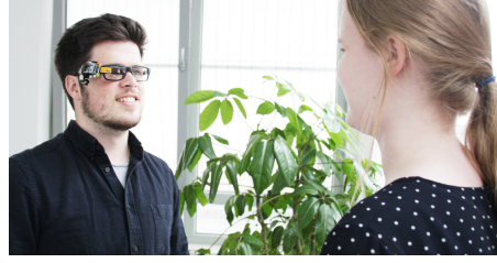
Figure 4: Left: simplified illustration of optical parameters used to calculate the distance between camera wearer and conversation partner. Right: working prototype consisting of a glasses frame with attached Vufine display, a Raspberry Pi Zero including camera and battery pack.
